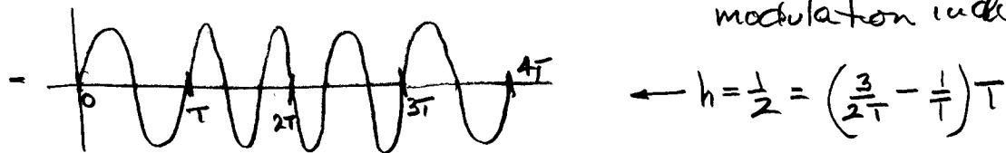
Any symbol of odd # of half-cycles reverses the starting phase.
