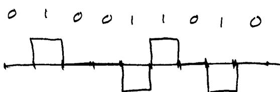
logic '1' sent with alternating polarity +1, -1
