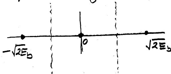
$$\Pr[\text{err} | "0"] = 2Q\left(\frac{\sqrt{2E_b}}{2\sqrt{N_0/2}}\right) = 2Q(\sqrt{\gamma_b})$$
