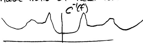
This causes the noise power to be exaggerated, so you lose SNR margin.
