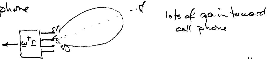
Now if interfering cell phones, must pick  $w$  to create nulls in those directions. Each such constraint reduces by one the number of degrees of freedom to max SNR.
