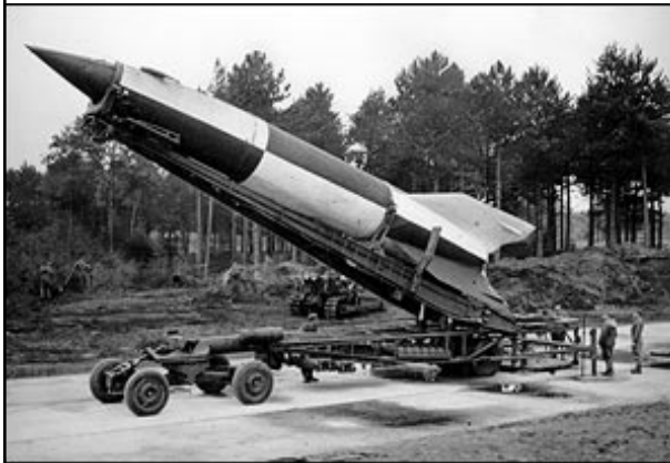
V2 (A4): First big liquid Rocket 25 Tonne Thrust, 200 Km range
