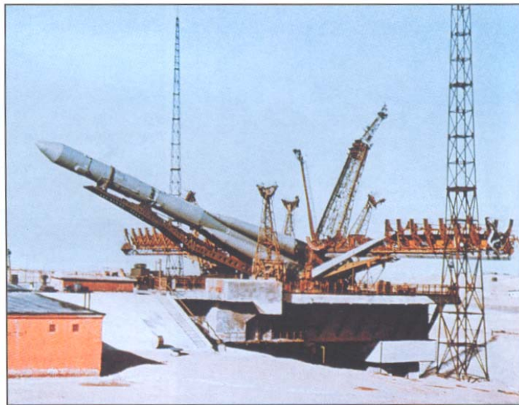
Russian Soyuz Booster being Erected
