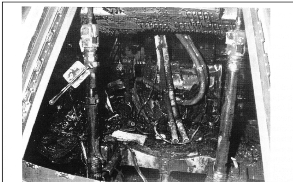
The interior of CM 012 (Apollo 1), showing the effects of the intense heat of the flash fire which claimed the lives of the three Apollo 1 astronauts, Grissom, White and Chaffee. Jan. 27, 1967 Apollo 1 fire: US program stops for 2 years
