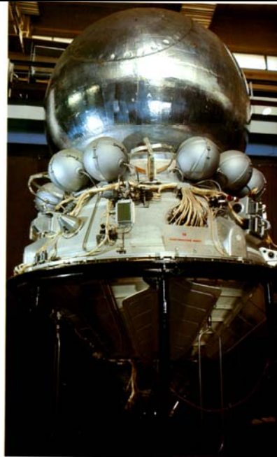
Above: The Vostok craft at assembly stage Note the oxygen and nitrogen life-support system bottle 'necklace'. Right: Vostok on display. Note the Kosmos-designated rocket.
