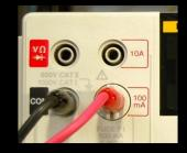
If the measured current is less than 100mA then move the red terminal to the 100mA range
