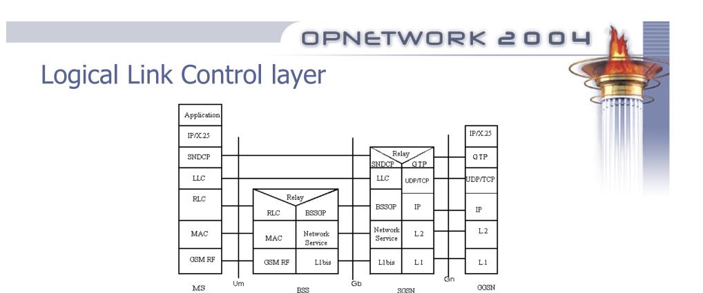
LLC, a sub-layer of layer 2 in the ISO 7-layer reference model, conveys information between layer-3 entities in the MS and the SGSN.
