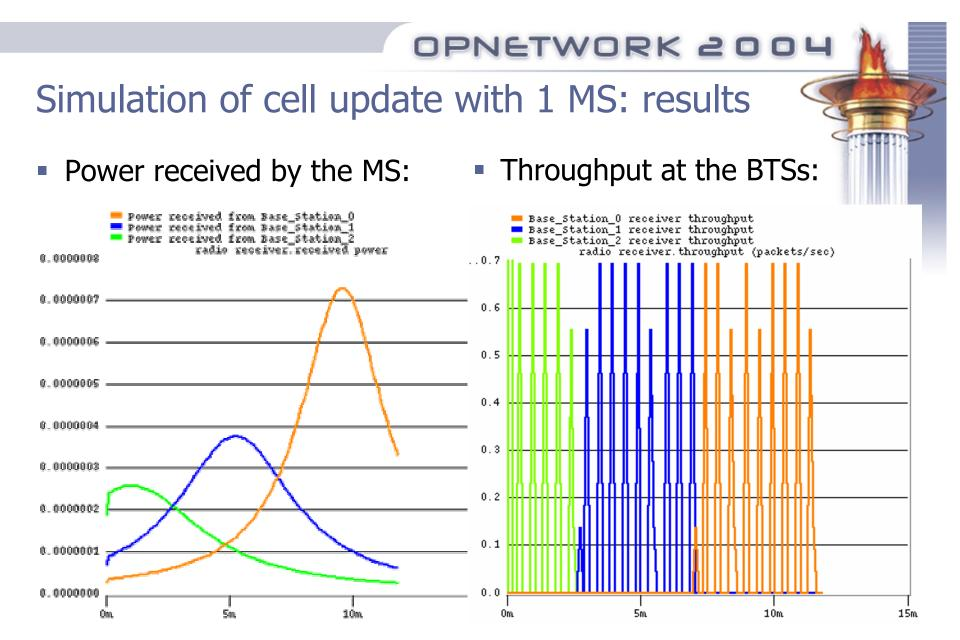
Simulation results verify that the cell update has been performed successfully.
