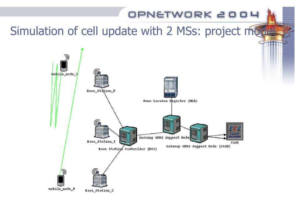
The MS mobile\_node\_1 moves between Base\_Station\_0 and Base\_Station\_1 only.
