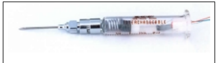
Figure 6. The integrated design of sampling mechanism consisting of passive preloaded coil spring and the latch mechanism based on the Concept 4.
