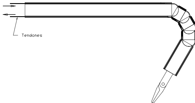
Figure 4: Tendon actuated multi-spherical joints design
