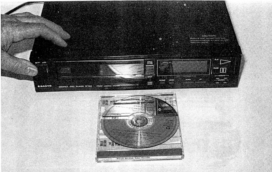
Fig. 2-1. The compact disc is only 120 mm in diameter with a large 15 mm center hole.
