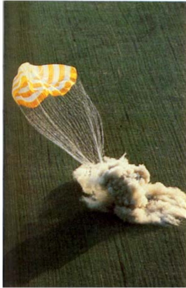
Above: The landing of a Soyuz descent module. The dust is not caused by the impact, but by the solid propellant retro-rockets firing.
