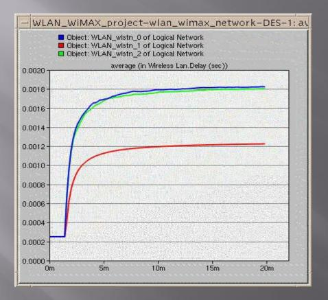
Delay of each workstations with WLAN Router
