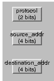
Figure 3 Request packet format
