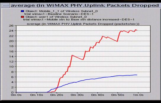
The graph depicts the uplink packets dropped when the modulation scheme for the Mobile Station is QPSK and the distance is increased to 30km. As we increase the increase not even QPSK being robust is not able mitigate the uplink packets dropped.
