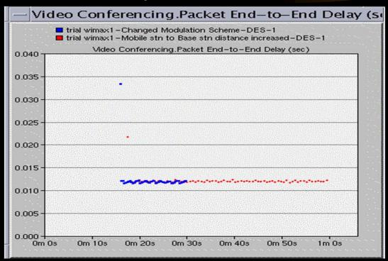
The graph depicts similar delay is achieved as the distance of the mobile stations is increased from 1km to 30kms and the modulation scheme is set to QPSK for the mobile stations. This implies that QPSK is Robust in nature.
