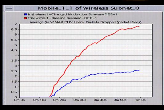
The graph depicts the uplink packets dropped when the modulation scheme for the Mobile Station changes from 64-QAM(baseline) to QPSK
