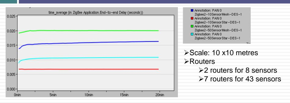
>Time taken for application packets to be transmitted from source to destination
