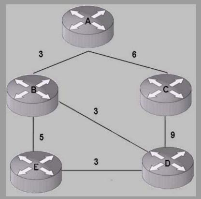
The link database for the above model is : [A, B, 3], C, 6], [B, A, 3], [B, D, 3], [B, 5], [C, A, 6], [C, D, 9], [D, C, 9], [D, B, 3], [D, E, 3], [E, B, and [E, D, 3].
