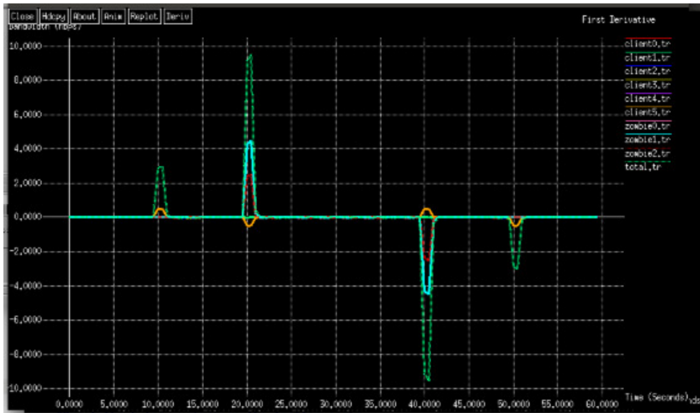
Figure 6: First derivative of the 'bandwidth vs. time' graph of a DDoS attack ( 0s < t < 60s ).
