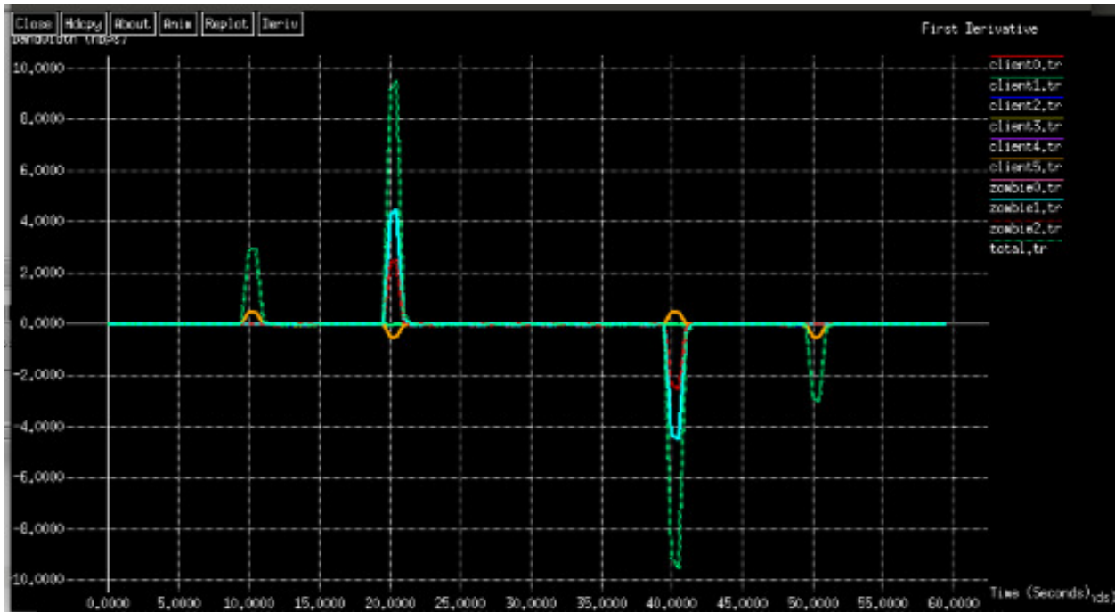
Figure 10: First derivative of the 'bandwidth vs. time' graph of a DDoS attack ( 0s < t < 60s ).
