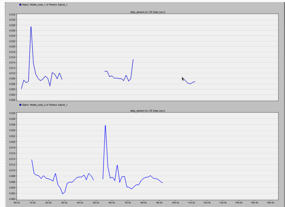
Delay of Two Mobile Nodes Traversing Three Base Stations
