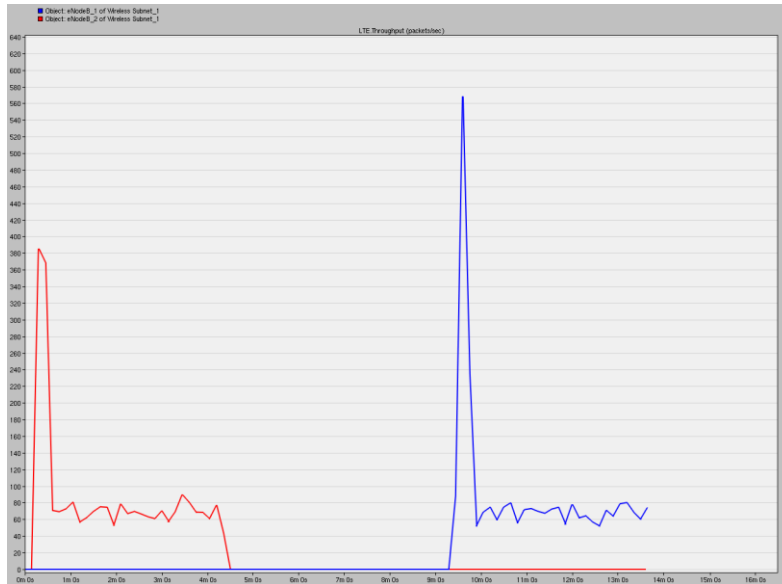
Figure 24- LTE network throughput of a mobile node traversing the cells from a 10MHz frequency base station to a 5MHz frequency base station.
