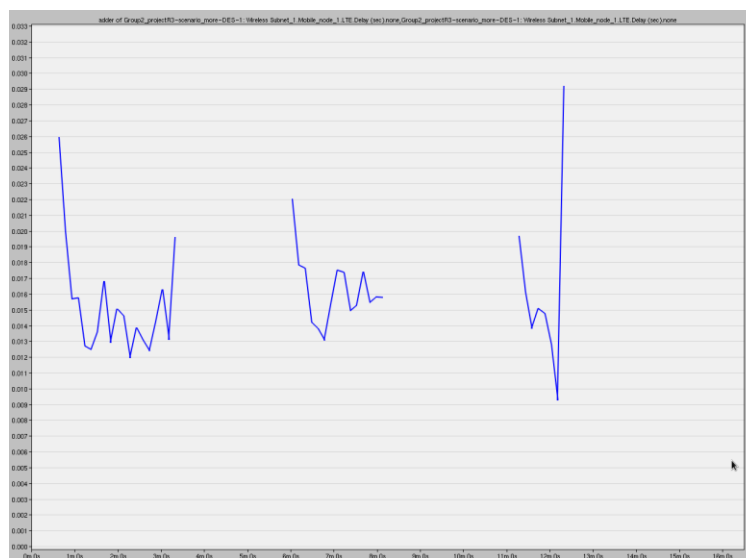
Figure 30- LTE network delay of a mobile node traversing the cells of three base stations with two 5MHz frequency and one 10MHz frequency.
