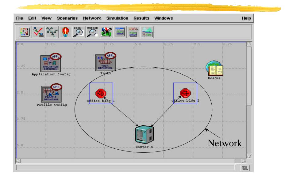
2 subnets, each has 1 access point, are connected by an Ethernet Router
