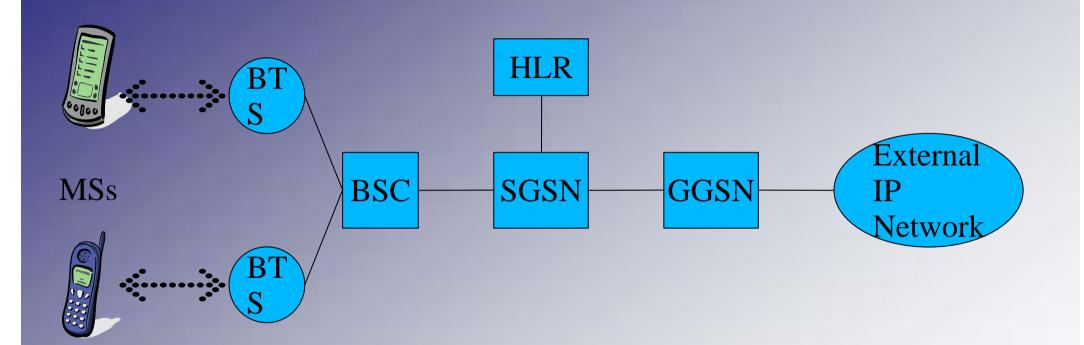
MS: Mobile Station BTS: Base Transmitter Station BSC: Base Station Controller HLR: Home Location Register SGSN: Serving GPRS Support Node GGSN: Gateway GPRS Support Node
