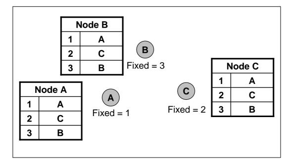
d. After the broadcast, node B's fixed interface switches to Channel 3 and each node's CUL gets updated.
