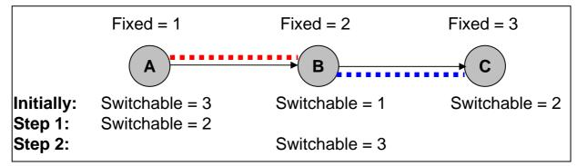
The sender adapts to the receiver by changing its switchable interface to the receiver's fixed interface
