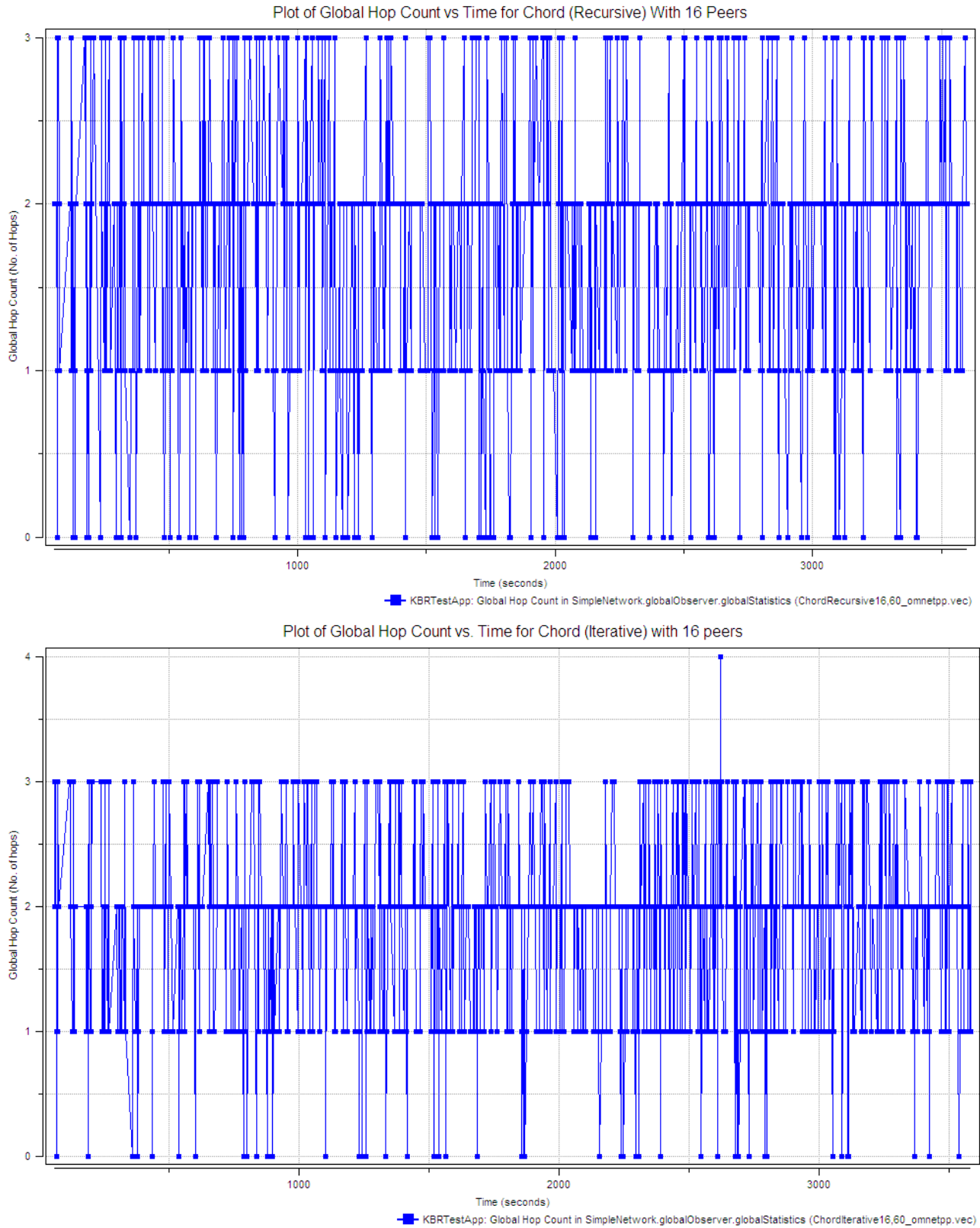
Figure 12(a) Global Hop Count vs. Time for Group 1 (top) and 2 (bottom) with 16 peers
