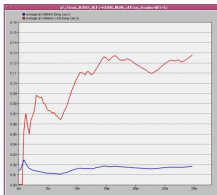
Figure 21: Global statistics delay of WiMAX and WiFi with 8 WiFi mobile users
