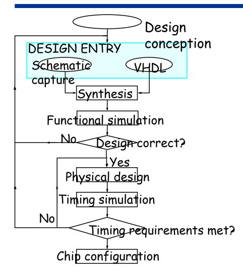
B&V: Figure 2.29. A typical CAD system.
