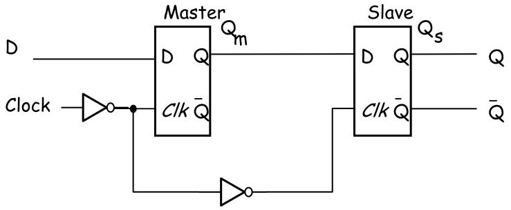
When Clk changes from 0 to 1, the value on D is copied to Q ("snapshot"), otherwise Q maintains its value
