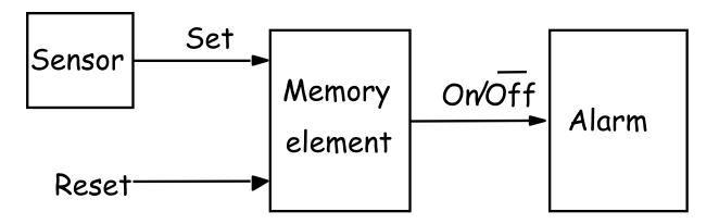
B&V: Figure 7.1. Control of an alarm system.
