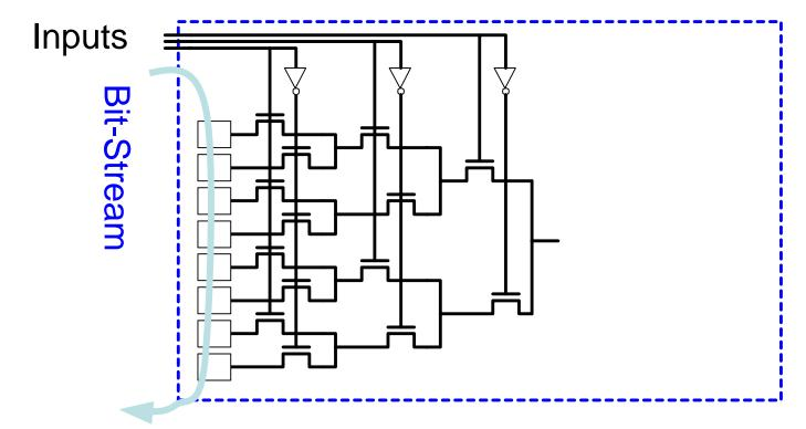
Function of each lookup table can be configured by shifting in bit-stream.
