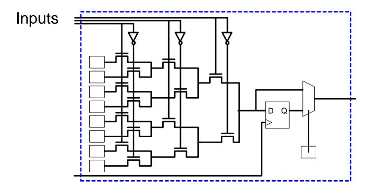
By adding a flipflop and multiplexer we can produce both registered and combinational outputs
