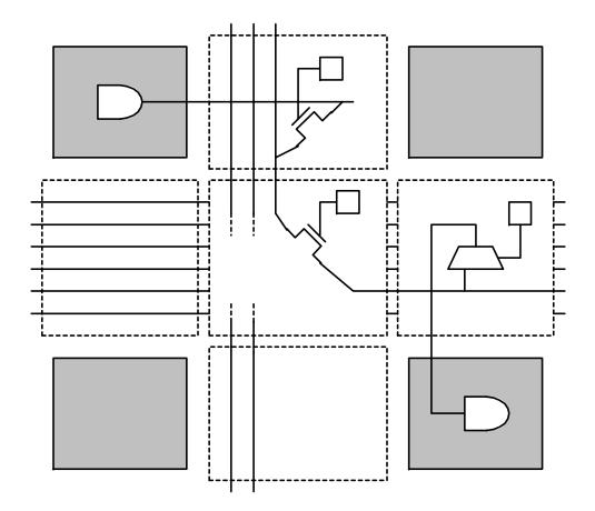
Connect Logic Blocks using Fixed Metal Tracks and Programmable Switches
