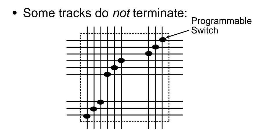
Connect using "Disjoint" pattern
