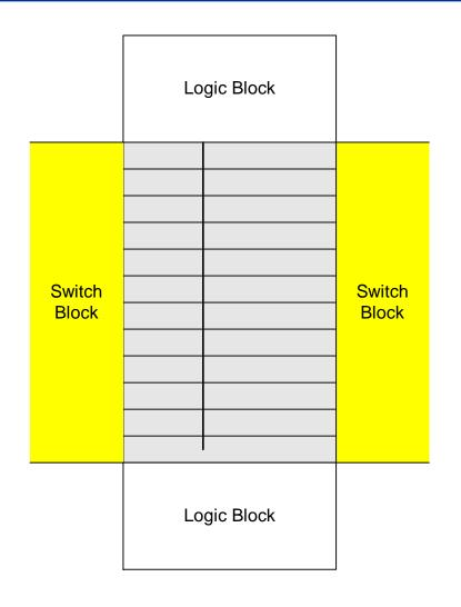
Each pin can connect to a subset of the tracks in an adjacent channel
