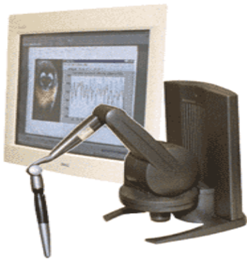
Fig. 3. Haptic device for force feedback.
