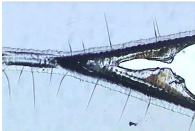
Fig.3. Partially released SU-8 in microchannel. Observe the stress cracks around the exterior of the microchannel.
